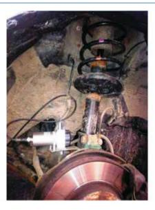
Fig. 2. On the left – on the test stand "Safeline 400/800" intended for measurement of shock-absorbers effectiveness. On the right – measurement of the car suspension travel
