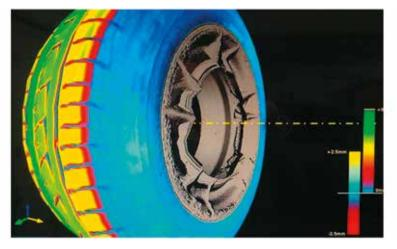
Fig. 5. Measurement of quantitative and qualitative parameters of a tyre using laser technique
