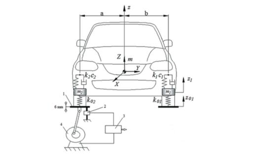
Fig. 1. A half-car model for dynamic analysis and principal mode of EUSAMA method (on the left side): 1 – pad of the plate, 2 – tension sensor, 3 – data processing, 4 – vibration generator
