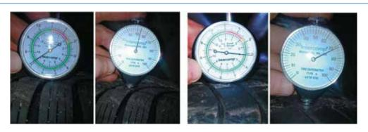
Fig. 3. Winter tyre tread depth and rubber hardness
